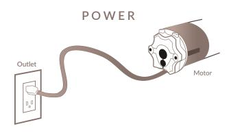
The Plug and Play motorized system uses a traditional 3 prong plug to draw power from a wall outlet. Each motor requires its own connection of 110 volt direct power.
